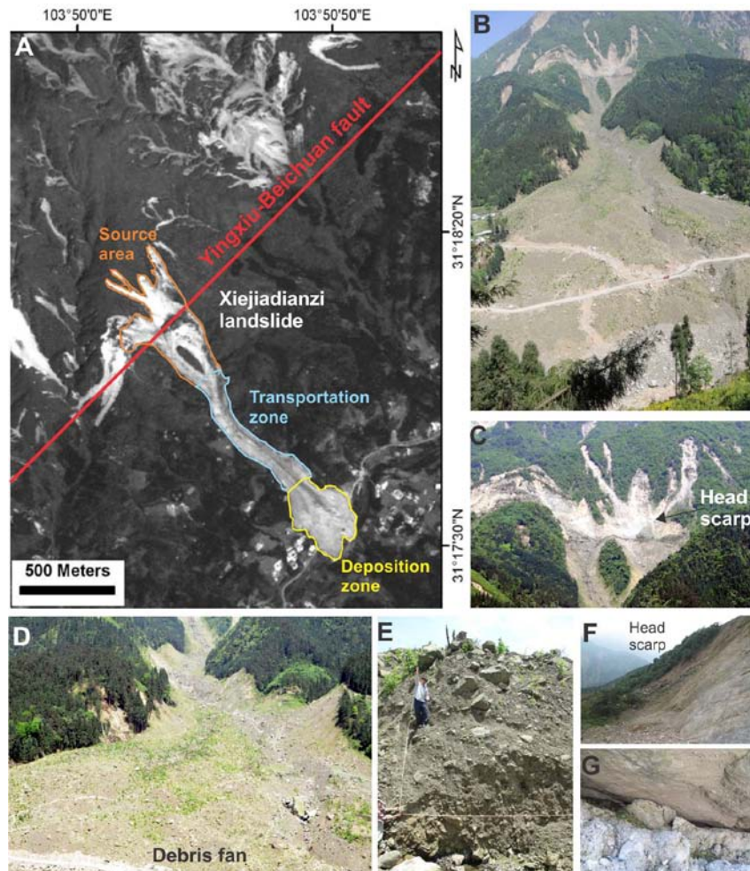
Figure 2.13 Xiejiadianzi landslide. A: ALOS PRISM Pan image of the Xiejiadianzi landslide; B: Overview photo; C: Source area; D: Depositional zone; E: Exposure of the deposits in the debris fan revealed by the valley incision; F: Head scarp, and G: Fine sediments under and mudline on a large block, indicating possible liquefaction phenomenon.
